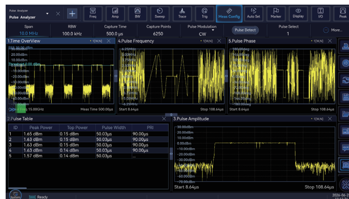
Multiple modulations in the pulse (linear frequency modulation, Barker code, etc.)
