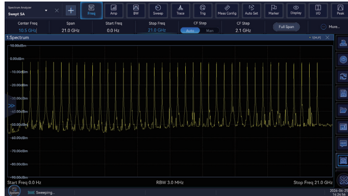
frequency-agile step changes of 0.5 GHz from 1 GHz to 20 GHz
