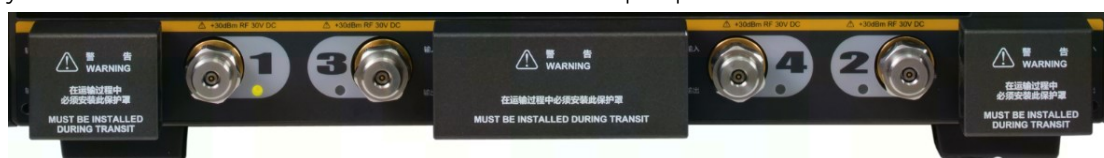
Figure 3.23 Test port of analyzer
