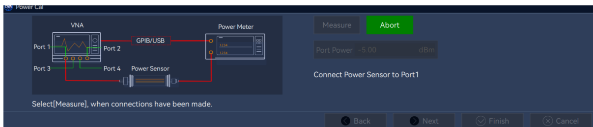
Figure 7.9 Source Calibration Measurement interface (with measurement in progress)
