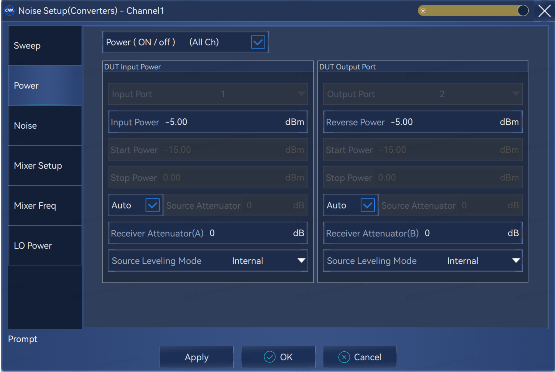
Figure 8.23 Converter noise figure measurement power tab
